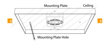
3 Align the mounting plate holes with the electrical box holes and mark four points onto the ceiling through the mounting holes.
