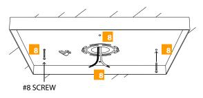
8 Secure the mounting plate to the anchors with the 4 provided #8 screws.
