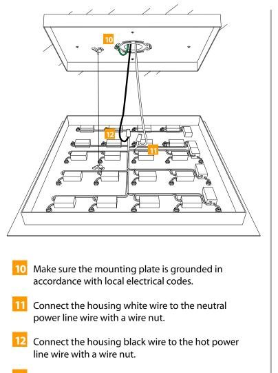
13 Place all wires and wire nut connections properly inside the housing.
