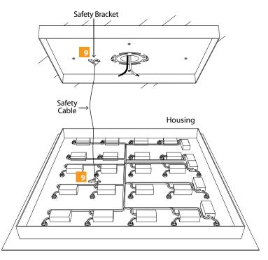
Insert one end of the safety cable into the mounting plate safety bracket and insert the other end into the housing safety bracket.
